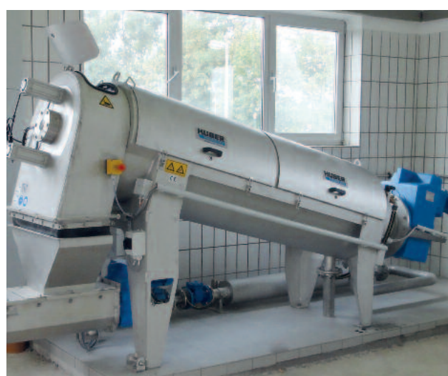
Stationary mounted screw press for 140 kg DS /h
