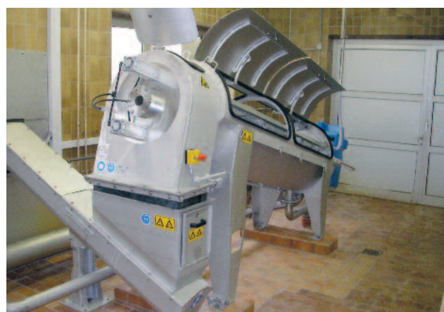
Complete size 440 installation with only a 12 m 2 footprint
