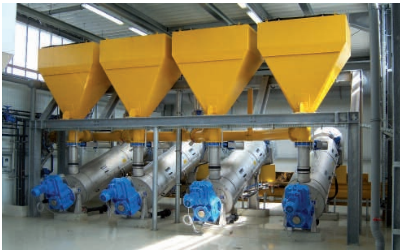
ROTAMAT® Screw Press RoS 3 Bio units with intermediate storage tank
