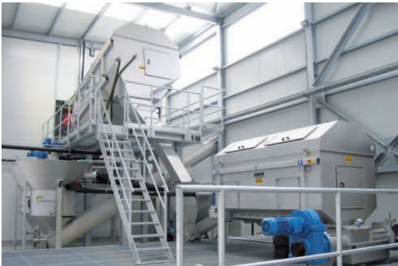
HUBER Wash Drum RoSF 9 with two subsequent HUBER Grit Washer RoSF 4 units, coarse material washer, ROTAMAT® Rotary Mesh Screen RoMesh® for organics removal and compaction
