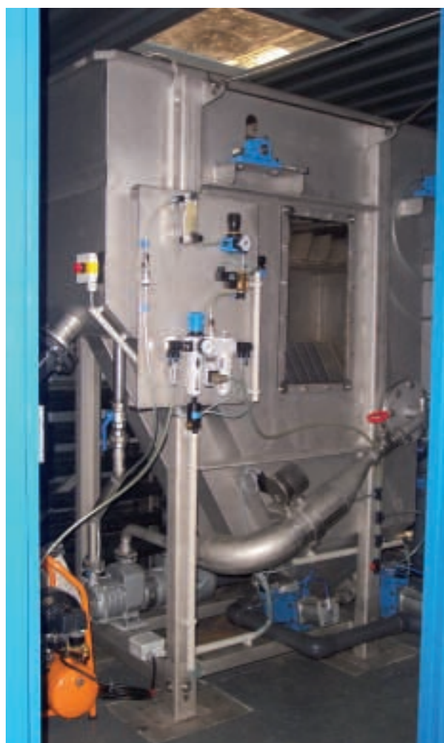
Dissolved Air Flotation test plant
