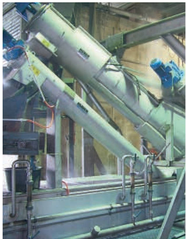
HUBER ROTAMAT® Complete Plant Ro 5 Bio and HUBER ROTAMAT® Screenings Compactor Ro 7 installed at RECYBELL, Boden
