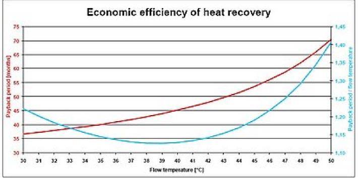
The blue curve describes the payback period / flow temperature ratio. The optimal operating point is achieved with a low payback period and high temperature within the heating circuit. The quotient of both values has therefore its lowest value at the optimal operating point. The diagram shows this value at approx. 39 °C. The optimal temperature for a heating plant with heat pump lies between 35 ° and 45 °. This fact is underlined by the figures provided by the diagram.
