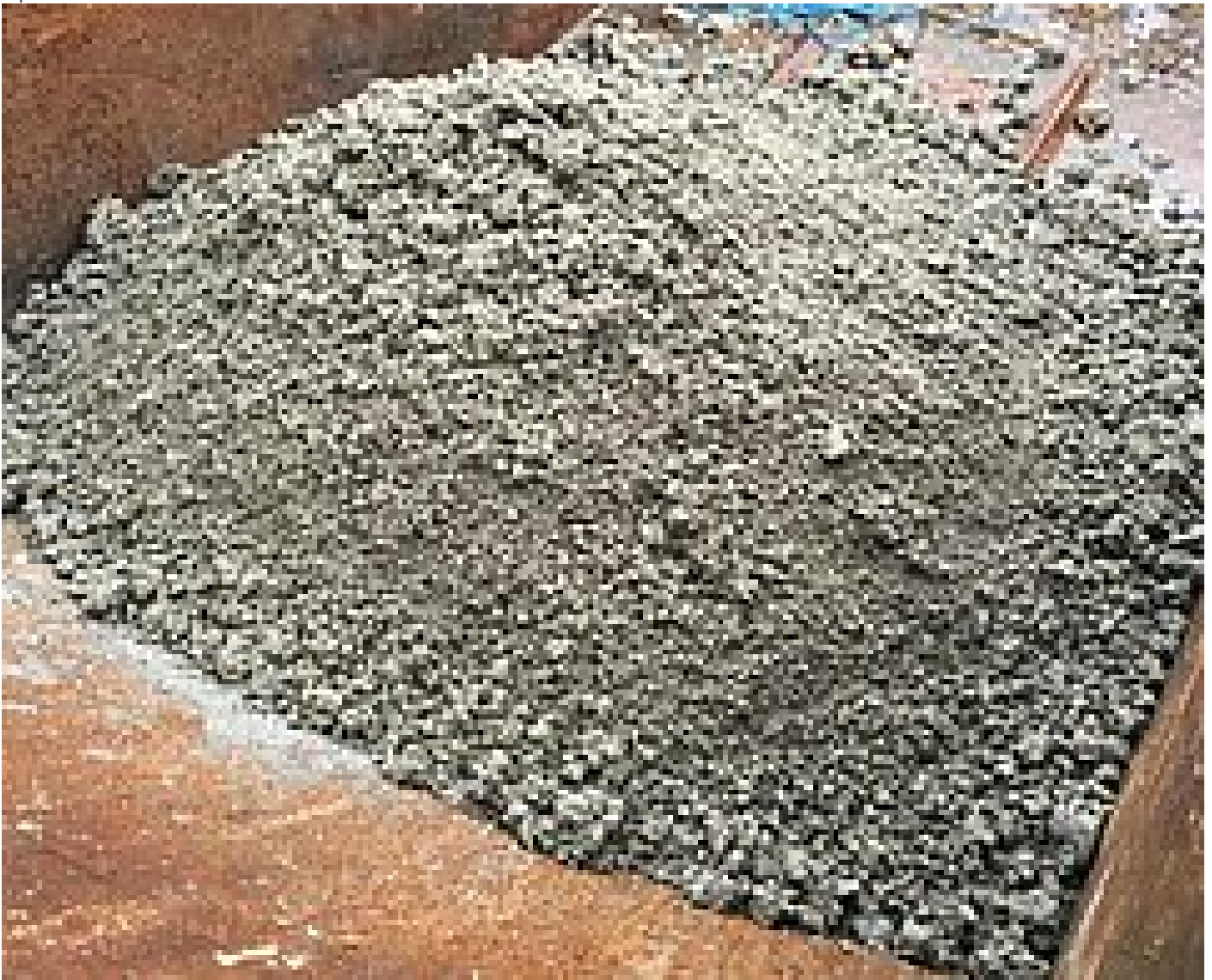
Dewatered sludge cake from the Q-PRESS®
